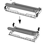
Remove the four green gears from the used film.
